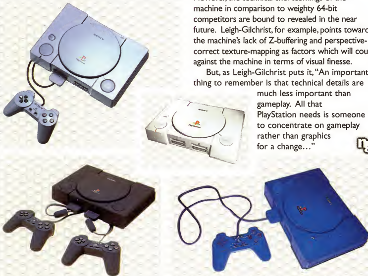
Sony has so far released four different versions of the PlayStation (from left): the standard grey model, the white Asia-only model (with enhanced MPEG playback), the programmable Yaroze, and the development blue machine
